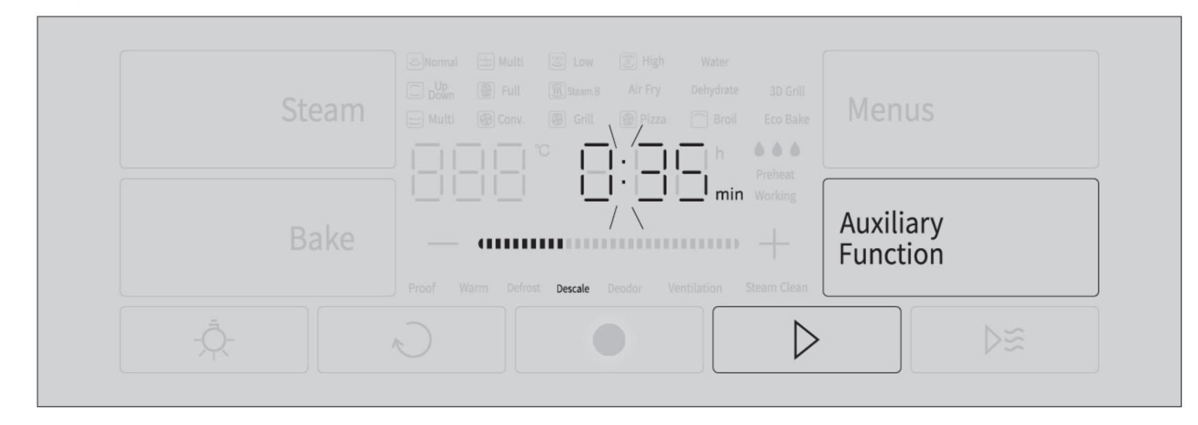
4. Descaling is completed. After the work is completed, the countdown reaches zero, with ten buzzers given.
