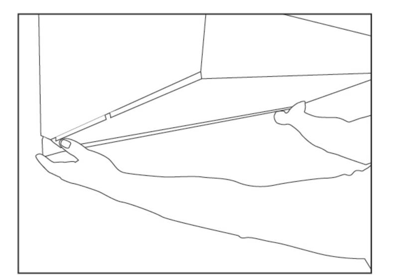
2. Touch the power button, and then the lighting button, open the smoke shield, and unplug the power plug. Hold the upper end of the grille with both hands and pull the locking tab downward to remove the grille. Immerse the oil cup and grille in warm water containing neutral detergent and wash them with a soft brush. After cleaning, install the oil cup and grille.
