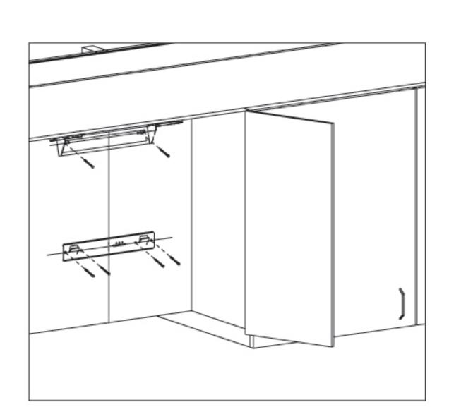
2) two cover hook screws (ST2.9 × 19 mm) can be used to fix it to the ceiling.(Applies only to purchased decorative cover components)
